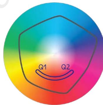
The transition is from Amber to Pink and in this case you pass through a Red that has the same saturation as the two end points as it is equidistant from the center of the circle. We move in an arc, not a straight line.
