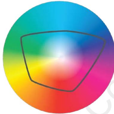
The addition of Amber offered slightly more colors, but not necessarily more light. Brightness is purely a matter of efficacy and the number of watts you pump into the luminaire. If you want a brighter light, just add more or bigger LEDs.
